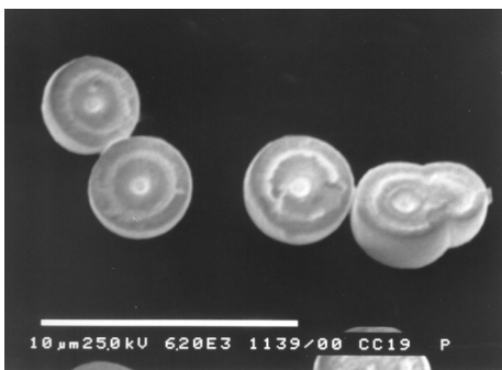
Fig. 8 Hollow spheres of fluoroapatite crystallised on the surface of the phosphate side from experiments at two times standard concentration (pH 7.4, Ca : F = 5 : 1, [Ca^{2+}] = 133 mM, [PO_4^{3-}] = 80 mM).
